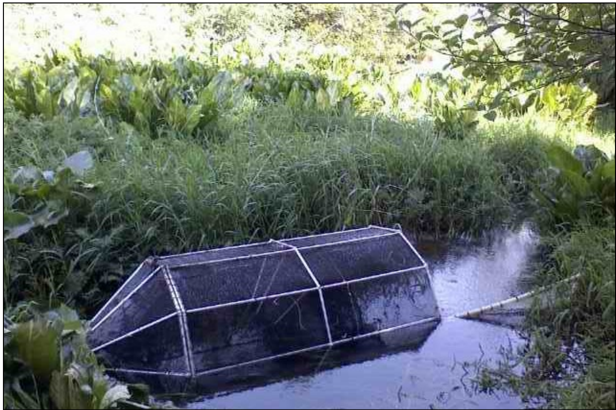
Smolt Trap Operation 2012—top photo shows a hoop trap fishing Cedar Creek (Elk River); bottom photo shows a hoop trap fishing Greene Creek (Sixes River). A local fabricator built the traps out of aluminum, using an existing ODFW trap as a template. The traps work by funneling fish through an inside cone that prevents them from swimming back upstream. To empty the catch the traps are pulled partially out of the water and the contents netted out.
